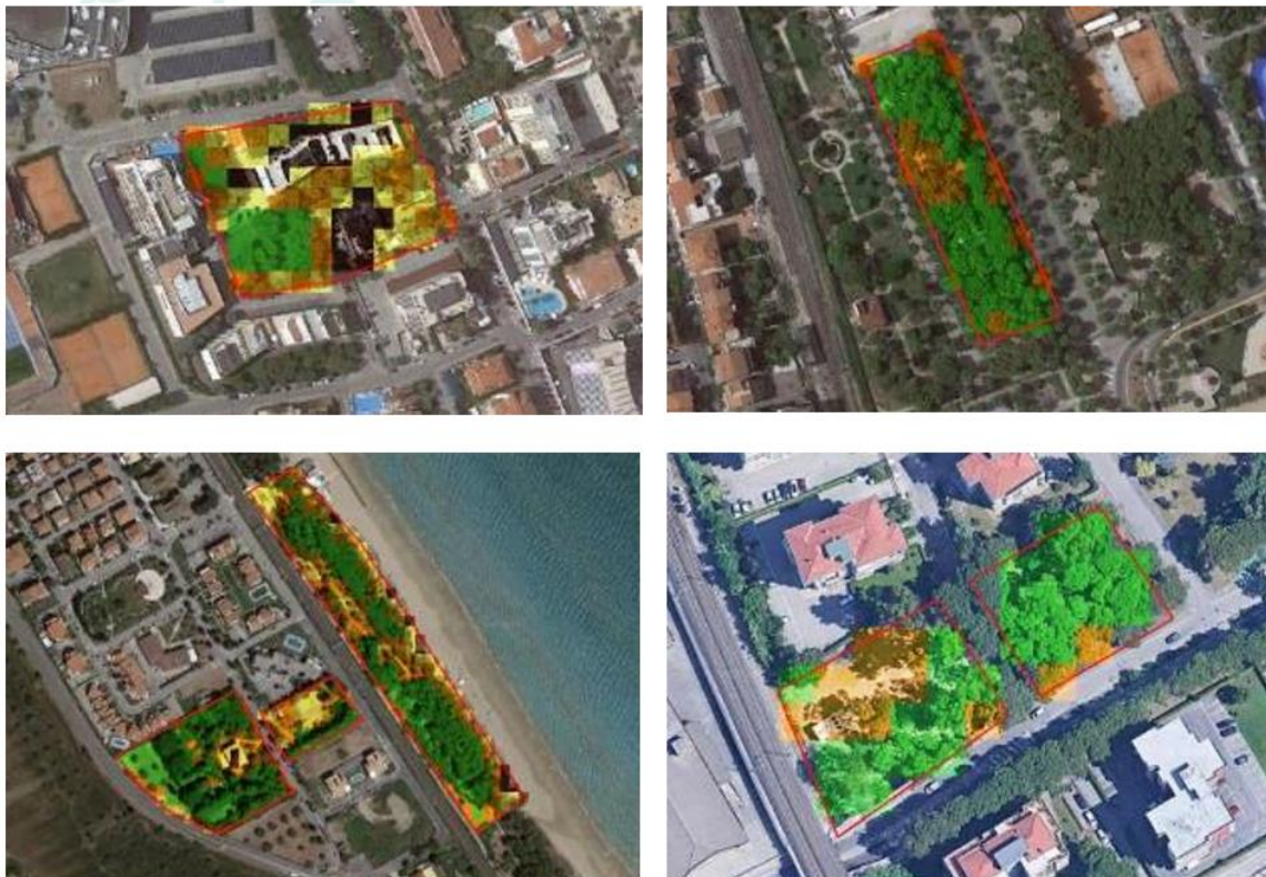
fig.25 Examples of overlapping of the SAVI index to the sample areas
